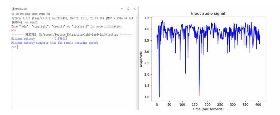
The output of the Entropy: the signal and the value of the minimum entropy.
