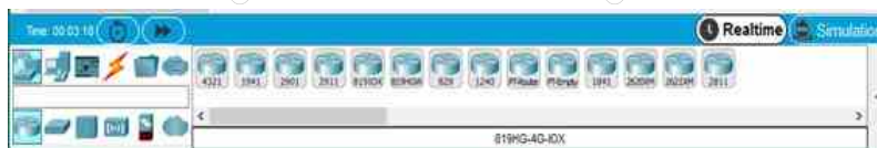
Figure 1.3: Top row = broad categories (Network Devices, End Devices, Connections), bottom row = subcategories (Routers, Switches, etc.).
