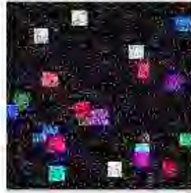
b. Median filtered image (3x3)
