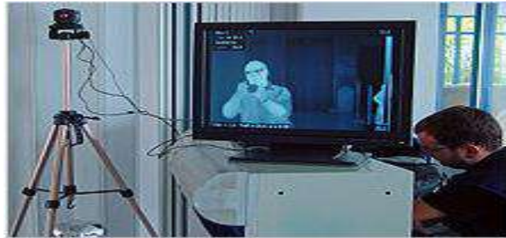
Thermal imaging camera & screen, in an airport terminal in Greece.
